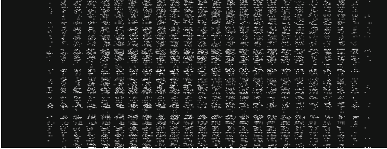
Fig. 2. Visualization of the first FC layer's sparsity pattern of Lenet-300-100.
