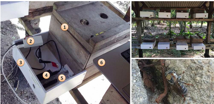
Fig. 1. Left: (1) Melipona fasciculata hive, (2) Intel Edison for RFID controlling and data storage, (3) PVC box for storing electronic items, (4) RFID reading antenna, (5) Plastic tube for bees' passage. Right-top: The 8 hives overview. Right-bottom: Bee with RFID tag attached to the chest.
