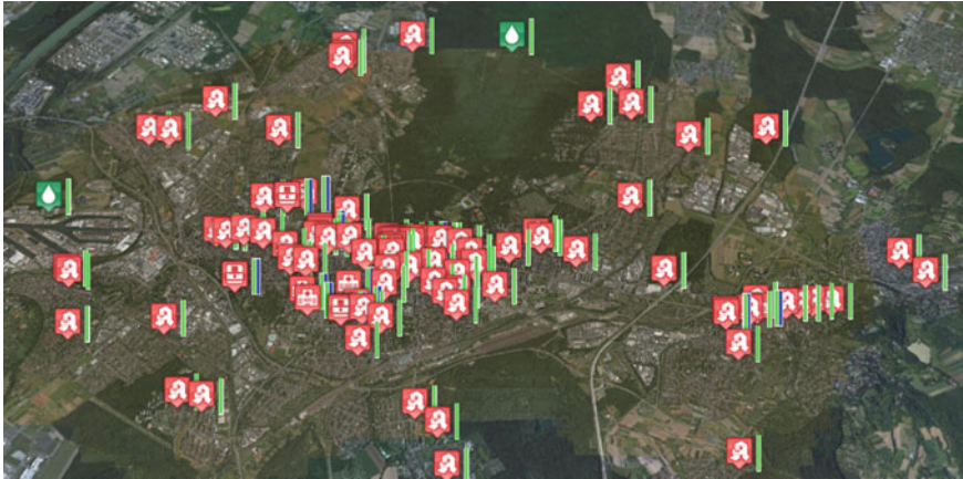
Fig. 16.4 An agent-based realization of some critical infrastructures of the city of Karlsruhe. The different icons indicate water supply, hospitals, pharmacies, and dialysis clinic. The green and blue bars indicate the state of the power respectively water supply of the according structure for the considered point in time of the simulation
