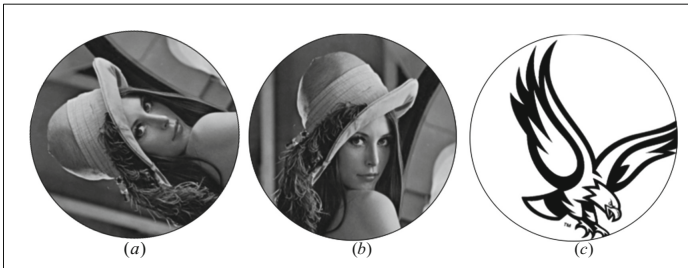
Fig. 4. Rotation attack. (a) The stego image attacked by rotation, (b) the stego image restored by the quantum image registration algorithm, (c) the watermark image extracted from (b).
