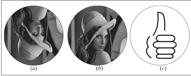
Fig. 6. Horizontal axisymmetry. (a) The stego image attacked by vertical axisymmetry, (b) the stego image restored, (c) the watermark image extracted from (b).
