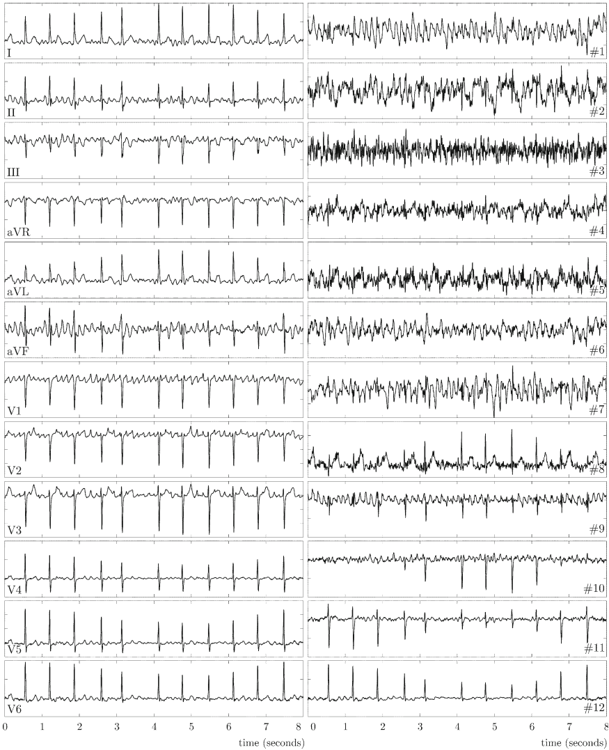
Fig. 5.18 f wave extraction using independent component analysis. a Original 12-lead ECG and b resulting independent components, displayed for increasing values of kurtosis (top to bottom). (Reprinted from [123] with permission)
