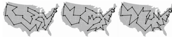
Fig. 2. The optimal k -robust TSP tour over all the U.S. state capital cities, for k = 1 (left), k = 2 (center), and k = 3 (right). The tours show greater regional coherence and more zigzags with increasing k .
