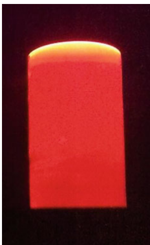
Fig. 1. The PS activated by the dibenzoilmethanate-Eu-1,10-phenanthroline europium complex under UV-irradiation
