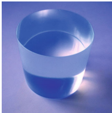
Fig. 9. PSD PS (25 mm diameter and 70 mm height) with 40% TBPPD
