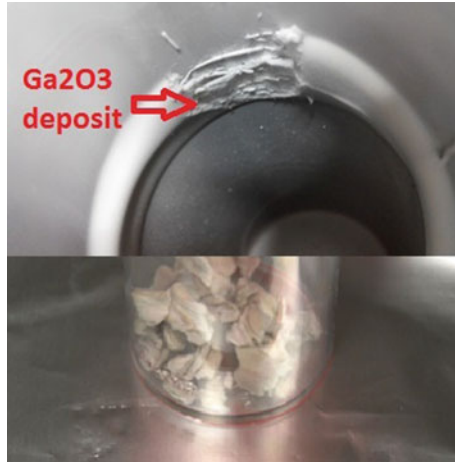
Fig. 9 Ga oxide deposited at the heat insulation after YAGG fiber growth by the micro-PD method. The lower photo represents the deposit collected into a test-tube
