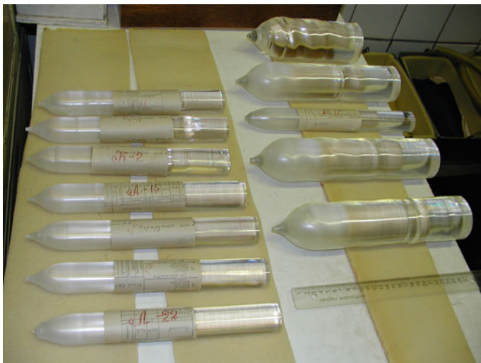
Fig. 3 Different types PWO ingots which were under production at BTCP since 1999 year
