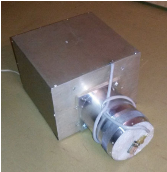
Fig. 11 Photo of the gamma-spectrometer used for the study of TGEs and for the search for gamma-flashes from lightning in Moscow region. GPS sensor is placed on the detectors head
