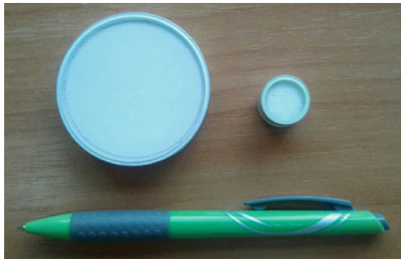
Fig. 15. {}^6\text{Li}(\text{Eu}) composite detectors dimensions 51 \times 2 mm and 12 \times 2 mm
