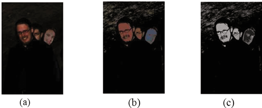
Fig. 5. (a) Forged image with the third person copy-pasted. (b) Illuminant map. (c) Distance map. Illuminant map and distance map clearly shows the third face as an inconsistent region [31] (Reprinted from Riess, C., Angelopoulou, E.: Scene illumination as an indicator of image manipulation. In: Information Hiding. vol. 6387, pp. 66–80 (2010) with permission from Springer).
