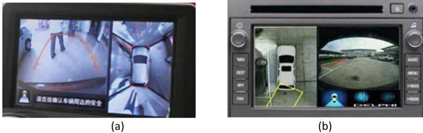
**Fig. 1.** The panoramic system of Nissan X-Trail and Delphi BEV Gen1.1, (a) Nissan X-Trail (2012), (b) Delphi BEV Gen1.1
