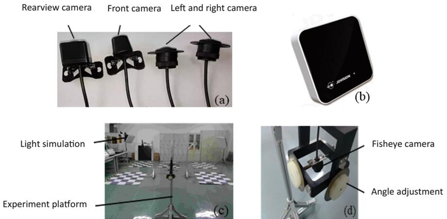
**Fig. 9.** Hardware platform of experiment, (a) Four way super wide angle fisheye camera for vehicle, (b) Video capture card, (c) Platform analog system, (d) Tilt angle adjusting mechanism
