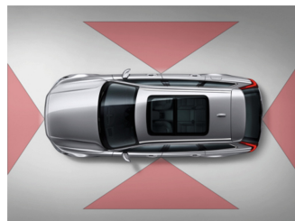
Fig. 1. Example fields of view of a multi-perspective camera mounted on a modern car.
