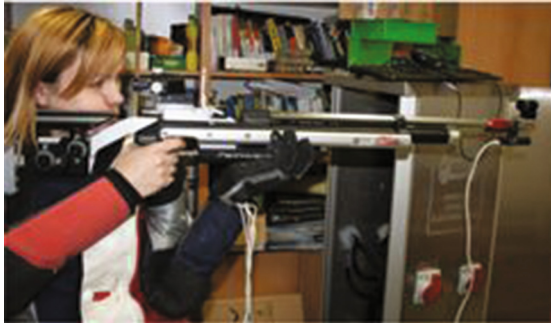
Fig. 4. Preparing of measurement in laboratory – shooter in standing position with air rifle. Sensor of SCATT system is attached on the end of the barrel.
