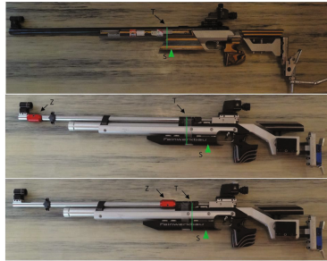
Fig. 8. Rifle setting. Above: sport rifle. Middel and bottom: air rifle. T – vertical axis of rifle center of gravity, S – support point, Z – additional weight.
