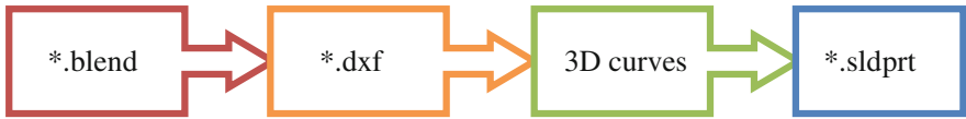
Fig. 6. The process of transfer of geometric data from Blender into the CAD system SolidWorks
