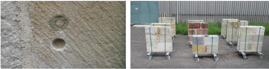
Fig. 1. (a) First from the left – The inserted cylindrical sample of Božanov sandstone after its primal Micro-CT analysis, (b) second from the left – experimental stone walls
