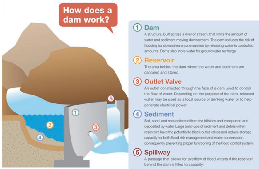
Fig. 7.1 Schematic diagram of a flood control dam describing different components (County of Los Angeles, Department of Public Works, www.lasedimentmanagement.com )
