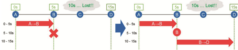
Fig. 5. Example of pedestrian trajectory interpolation. Without interpolation, a beacon cannot be tracked until the signal from the beacon could be observed again. By trajectory interpolation, the system can track the beacon continuously, even if the signal from the beacon could not be observed for a while.
