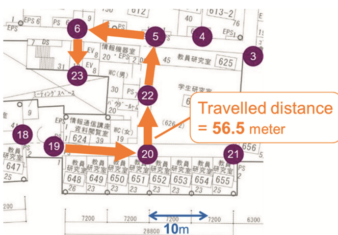
Fig. 3. Error reduction with estimated walking speed. Since a device has been estimated as having traveled from AP19 to AP23 (56.5 m) in 5 s, the latest position estimate (AP23) is eliminated.
