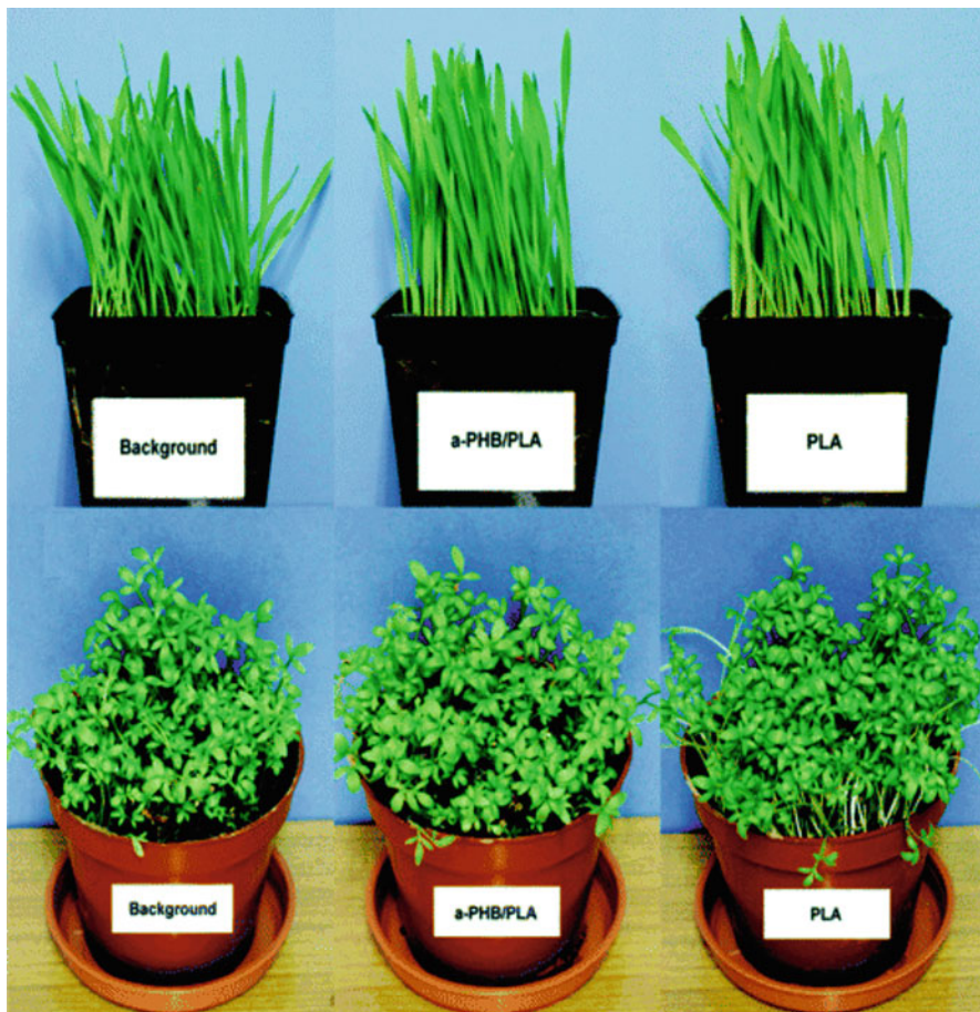
Fig. 8 Ecotoxicology test, growth of barley ( upper images ) and cress in soil after 183 days of degradation of aPHB/PLA and PLA films (Adapted with permission from Rychter et al. [82] Copyright, 2006, American Chemical Society)
