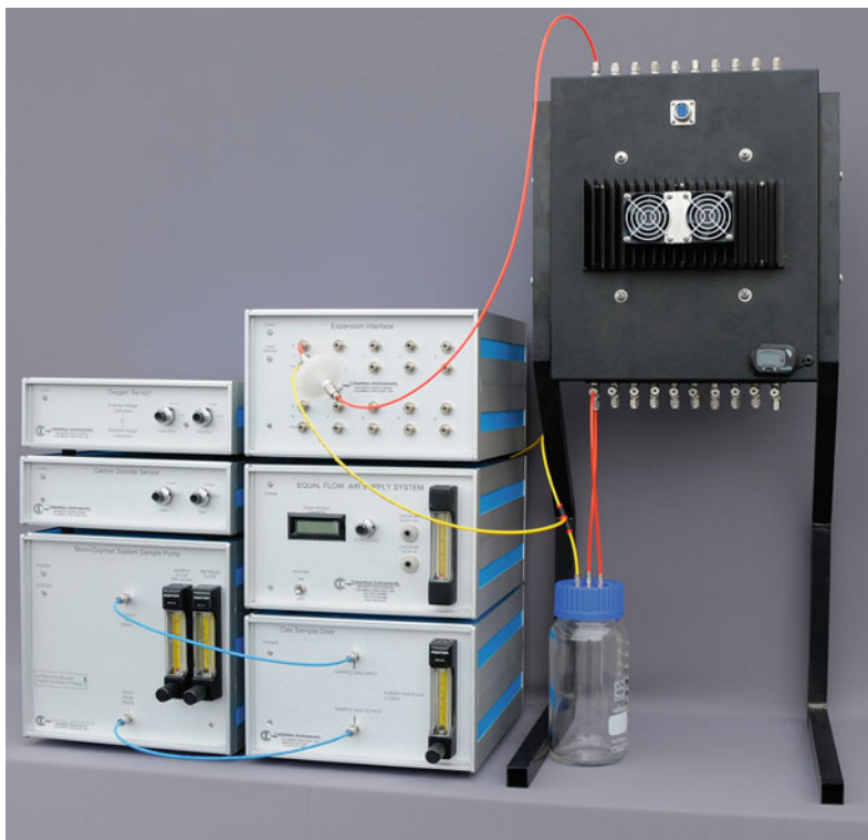
Fig. 7 Micro-Oxymax respirometer (With permission, Copyright (2017) Columbus Instruments International)
