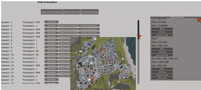
Fig. 7. The evaluation menu including the visualization of a participant's path on a map of the city. The menu also provides basic information about the path and the option to export the data collected by the different sensors.
