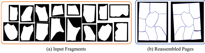
Fig. 6. Simultaneous reassembly of front and back of sheet 2, from dataset [11]. (a) Input: 8 fragments, both front and back sides scans. (b) Reassembled pages.
