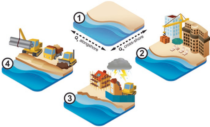
Fig. 1 Schematic of a developed barrier coastline as a coupled human–landscape system. (1) Natural processes of wave-driven sediment transport ( Q_s ) drive physical coastal changes in space and time; (2) development capitalizes on economically viable coastal real estate; (3) chronic or event-driven natural hazards damage coastal development and infrastructure, prompting (4) interventions to mitigate or prevent damage in the future. Such interventions modify the physical landscape, altering sediment fluxes in (1), pushing the cycle to iterate. Reprinted with permission from Elsevier from Lazarus et al. (2016), An evolving research agenda for human–coastal systems. Geomorphology , 256, 81–90
