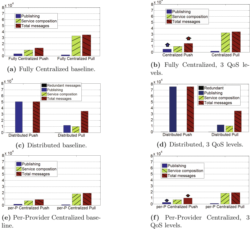
Fig. 5. Message overhead for all coordination models under two different setups.
