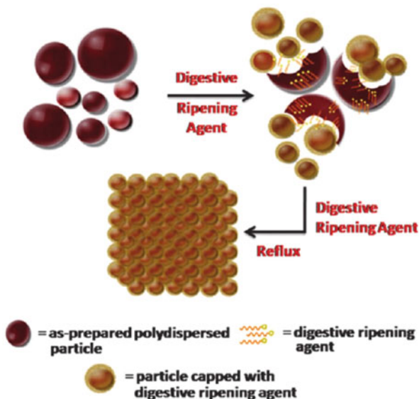
Fig. 2.5 Diagram showing the role of digestive ripening agent in the process (Figure reproduced with permission from [10])
