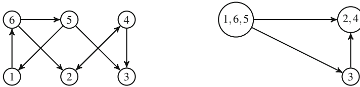
Fig. 1.5 An example of graph G (left) with its condensation graph \mathcal{T}(G) (right)
