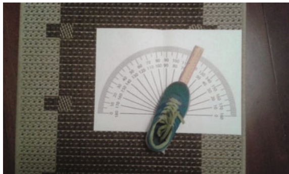
Fig. 11.9 The known FPA measured applying a protractor is used in defining reference angle FPA_{ref}
