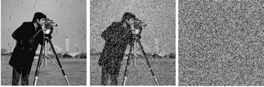
Fig. 3.8 The cameraman image transmitted by Alice and received by an eavesdropper: on the left, with no coset coding, in the middle with one bit of randomness, and on the right with two bits of randomness
