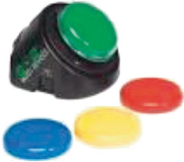
Fig. 17 Simple communicator: Go Talk (source: http://klik.com.br ) [39]. The simple communicator can be used to call for attention, for social interactions, for participation in activities, and to establish cause and effect
