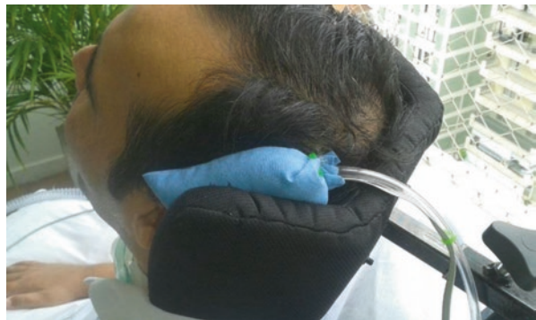
Fig. 22 Emergency call system adapted to a wheelchair, with a bell activated by a discreet cervical movement. It can be used as a trigger to be adapted to the computer
