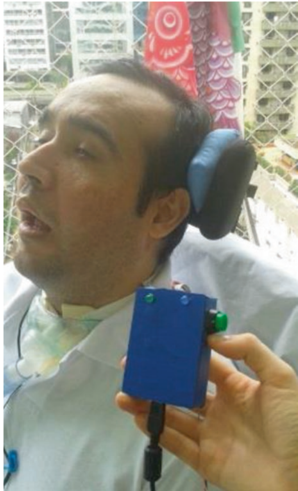
Fig. 21 Emergency call system adapted to a wheelchair, with a bell activated by a discreet cervical movement. It can be used as a trigger to be adapted to the computer
