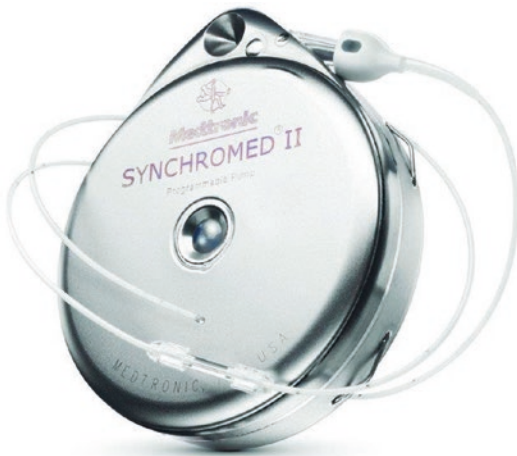
Fig. 25.1 SynchroMed II pump with 20 cc reservoir, 19.5 mm in thickness (also available with a 40 cc reservoir, which is 26 mm thick), and two-piece radiopaque Ascenda catheter system that has increased resistance to kinking, cuts, occlusions and leaks when exposed to tensile and compressive forces compared to a regular silicone catheter as a result of a thermoplastic polyethylene terephthalate braid and a polyurethane outer jacket covering the inner lumen of the silicone tubing. The peristaltic pump propels the medication from the reservoir to the catheter port that is connected to the catheter system leading to the intrathecal space. The pump requires replacement generally every 7 years because of the built in battery life span. The central port is accessed during baclofen refills with a 22-gauge Huber-type needle. The side port is designed to be accessed with a 25-gauge needle, usually for diagnostic purposes (photo used with permission, © 2016 Medtronic)
