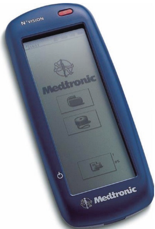
Fig. 25.2 Medtronic N'Vision® hand-held wireless portable programmer device (model 8840) for the SynchroMed II programmable baclofen infusion system (photo used with permission, © 2016 Medtronic)
