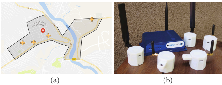
Fig. 1. LoRa deployment in Kikwit: (a) Range testing area; (b) LoRa gateway and fridge sensor devices
