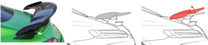
Fig. 11. Manually adjustable rear wing
