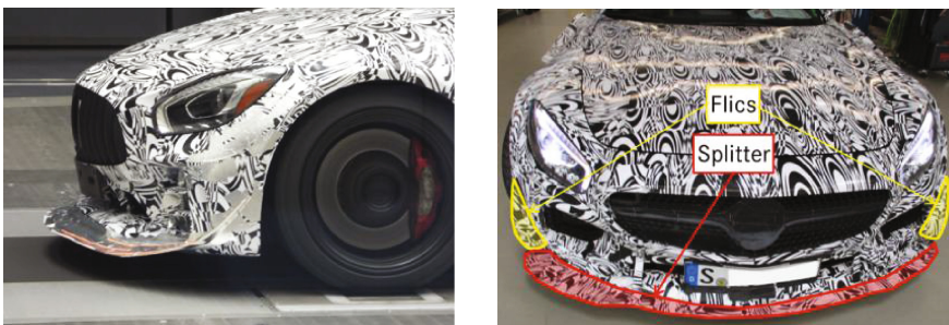
Fig. 6. Splitter proportions and flics to generate similar frontal lift ( C_{LF} ) as the active aero system on the underbody
