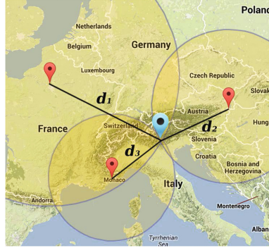
Fig. 2. Triangulation for specifying the physical location of a host by knowing the physical locations and distances from other nearby hosts.
