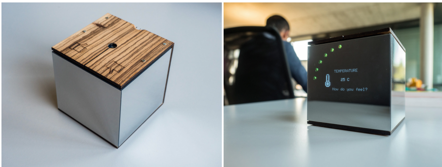
Fig. 2. ComfortBox is an interactive research tool designed to facilitate data collection in lab and in-situ comfort studies. The physical design is intended to help blend into the desktop setting and stay in the periphery of attention when not used.
