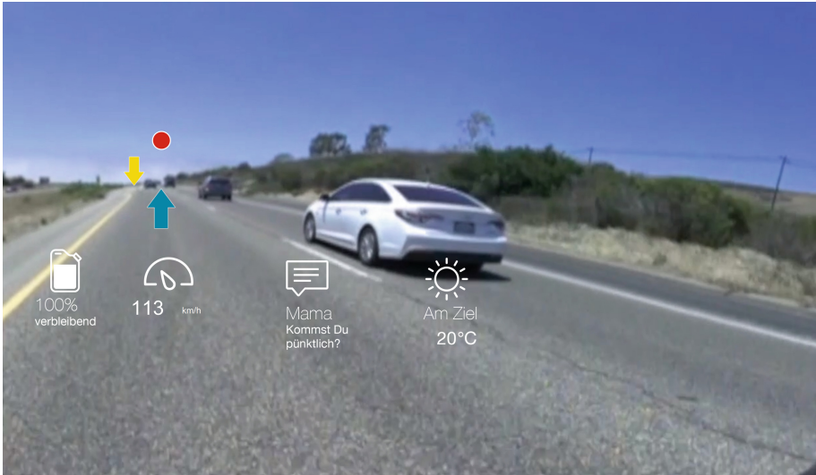
Fig. 2. An example view of the driver. The driving simulator software runs an adjusted version of the ConTRe task and footage of real driving with superimposed HUD content.
