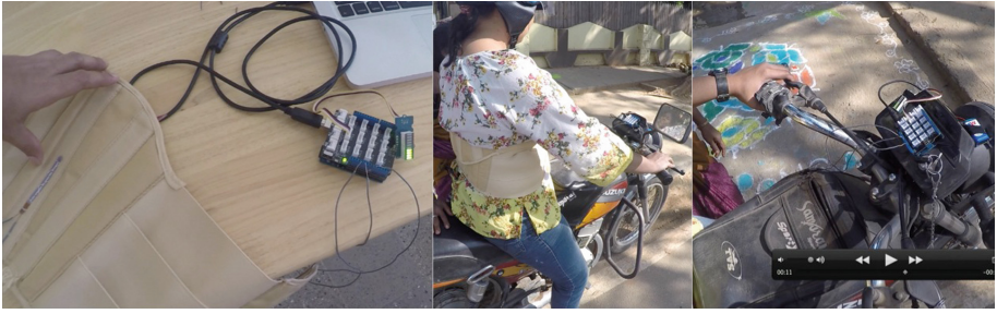
Fig. 3. ReRide interactive sketch. rider with the belt. The display next to speedometer
