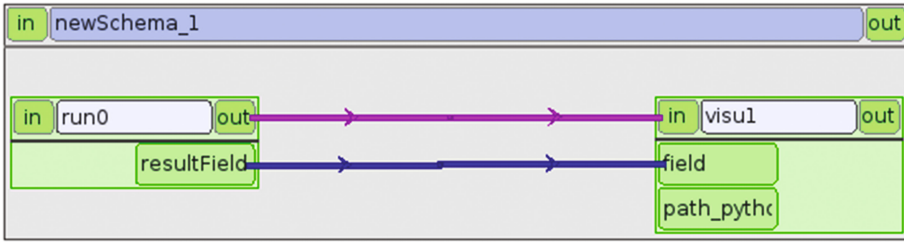
Fig. 3. Using visualization in a simple computation workflow, a solver (left node) is connected to a visualization service (right node).
