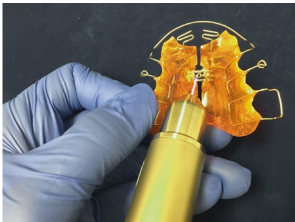
Fig. 18.1 Antimicrobial efficacy of CAP on removable orthodontic appliances. CAP is effective in destroying biofilms on acrylic baseplates and could therefore be a useful addition to current oral hygiene regimes. (Plasma source pictured: kinPen med, Neoplas tool, Greifswald, Germany)
