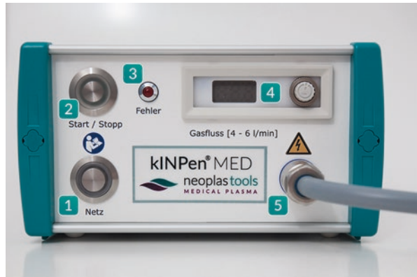
Fig. 32.5 Base unit with 1 power switch, 2 start/stop key, 3 error display (LED), 4 gas flow control 5 supply tube for the handpiece
