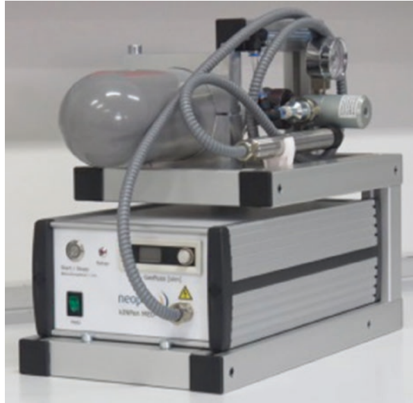
Fig. 12.21 kinpen Med mobile pocket for outpatient CAP therapy of patients with implanted heart support systems
