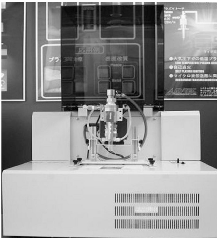
Fig. 13.3 Microwave Atmospheric pressure plasma device APTN-150 (Adtec Plasma Technology Co., Ltd)
