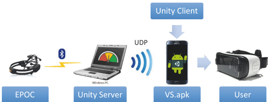
Fig. 3. Devices and software needed in Virtual Sophrologist System
