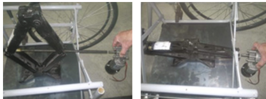
Fig. 9. Mounting and fixing the Car Jack, raising and lowering the engine position
