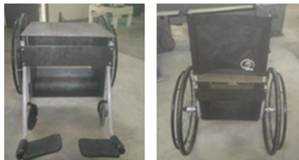
Fig. 10. Picture of seat basis structure and wheelchair assembled
