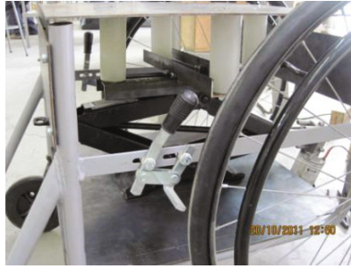
Fig. 11. Photo of detail of fixing of the structure of lifting and lowering system.
