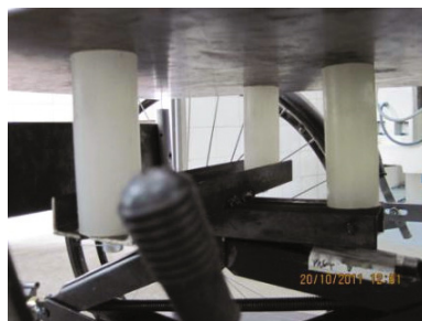
Fig. 13. Photo of the detail of seat fixing in the lifting and lowering system
