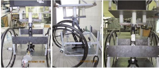
Fig. 17. Picture of details of lifting and lowering system
