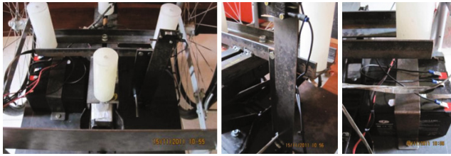
Fig. 18. Detail photo of battery fixing and end of stroke system
