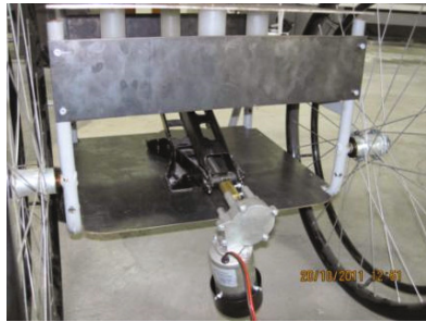
Fig. 12. Photo of engine fixing on Car Jack
