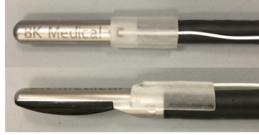
Fig. 1. Custom-designed EM tracking mount on the LUS transducer.
