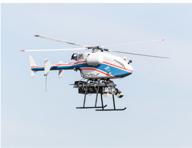
Fig. 1. One example UAS of the DLR Unmanned Aircraft Fleet: SuperARTIS, a dual rotor configuration vehicle, shown with complete flight computers and sensor setup.
