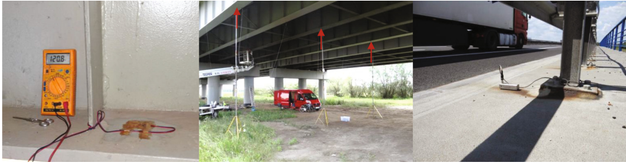
Fig. 5. Exemplary location of different types of measuring sensors in span 7–8: (a) strain gauge at point 00, (b) LVDT sensors at points 07–09, (c) accelerometer at point 10R
