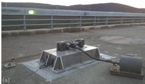
Fig. 2. (a) Eccentric mass shaker on the dam; (b) Generated excitation force.
