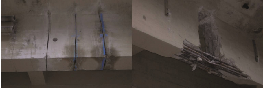
Fig. 6. Artificially damaged beams. The cuts introduced progressively during the tests, along with the damage in the centerline of the span.
