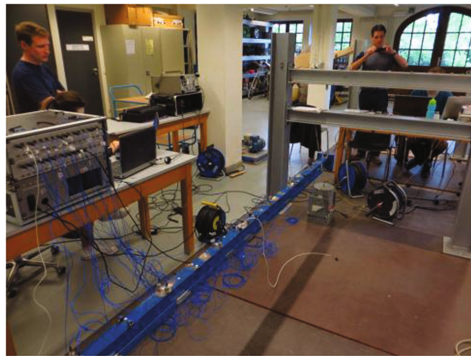
Fig. 4. Instrumented steel beam.
