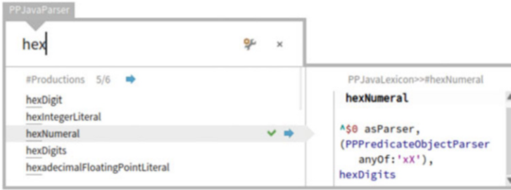
Fig. 8 Using Moldable Spotter to search for productions containing the word “hex” in a parser for Java code
