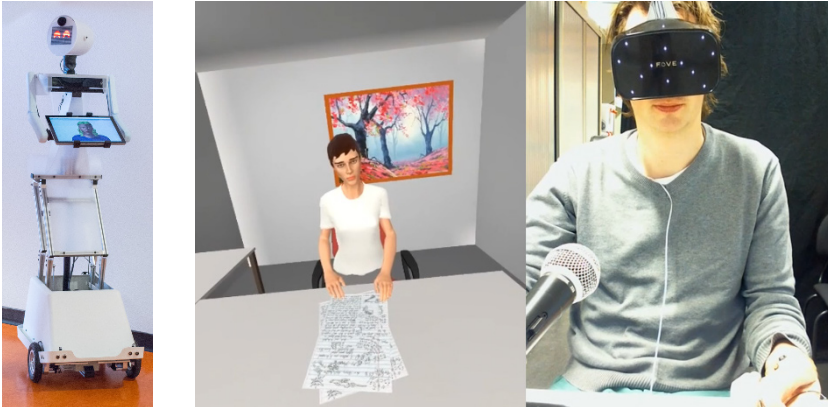
Fig. 2. The R3D3 robot (left) with a mixed-modality agent and the Moral Competence Training experiment setup in immersive VR (right)
