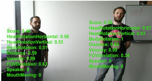
Fig. 3. Features and engagement scores shown on the Kinect stream
