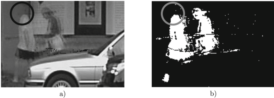
Fig. 4. Visual example of camouflage artifacts in background subtraction based algorithm: (a) frame 25 of Traffic sequence, (b) foreground mask.
