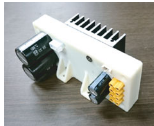
(b) Bottom side view of the multirotor MUAV. (c) Voltage step-down converter
