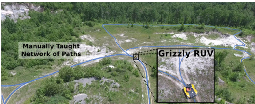
Fig. 1 A Grizzly RUV deployed with an autonomous path-following algorithm navigating a 5 km network of manually taught paths. Applications that rely on repeated traversals of constrained paths will greatly benefit from such algorithms: such as mining, agriculture, and patrol robots. In order to be useful for such applications, autonomous path-following algorithms will need to be able to cope with large-scale maps, and appearance change over long periods of time. Using a novel multi-experience localization and mapping method, the robot pictured above autonomously traversed over 140km over two weeks, experiencing significant appearance changes in the environment
