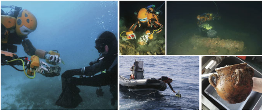
Fig. 11 Ocean one deployed in Toulon, France. Left: collaboration with a diver at 15 m depth. top center/right: O_2 fetching a vase and dropping it into the collection basket. bottom center/right: researchers collecting the floated basket, Catalan vase on deck showing its acquired biofilm. (Photos courtesy of Frederic Osada and Teddy Seguin, DRASSM/stanford university)
