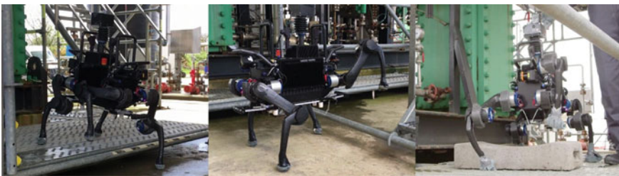
Fig. 8 ANYmal uses the Free Gait motion control architecture [4] to negotiate known (left and middle) and unknown (right) obstacles. For known obstacles we generated a database of parameterized motion definitions. Unknown obstacles are negotiated by selecting safe footholds from the environmental mapping and optimizing the body motion and posture
