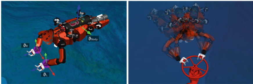
Fig. 4 Left: Task specification. Every task is associated with an operational-space \vartheta_{\text{Task}} , illustrated by the cartesian coordinate frames. The manipulation task consists of \vartheta_{\text{L}} and \vartheta_{\text{R}} , the six-dimensional spaces of the left and right hand—three coordinates for the frame origin (purple sphere) and three for the frame’s orientation. These spaces are controlled directly by the manipulation task, which is the only task receiving control inputs. This abstraction allows for unified motion and force control that is agnostic of the robot’s morphology. The body’s operational space \vartheta_{\text{Body}} is controlled by the Posture task such that it autonomously follows the hands. Right: Null-space of the manipulation task. The kinematics of O_2 are modeled with 20 DoF. The manipulation task occupies 6 DoF for each of the two arms. The remaining eight are controlled by the posture tasks. Here, O_2 performs a manipulation task on a red valve. The null-space is illustrated by various postures that leave the manipulation task variables (position and orientation of the white hands) undisturbed. This eight-dimensional posture can be used to execute the task in an optimized manner
