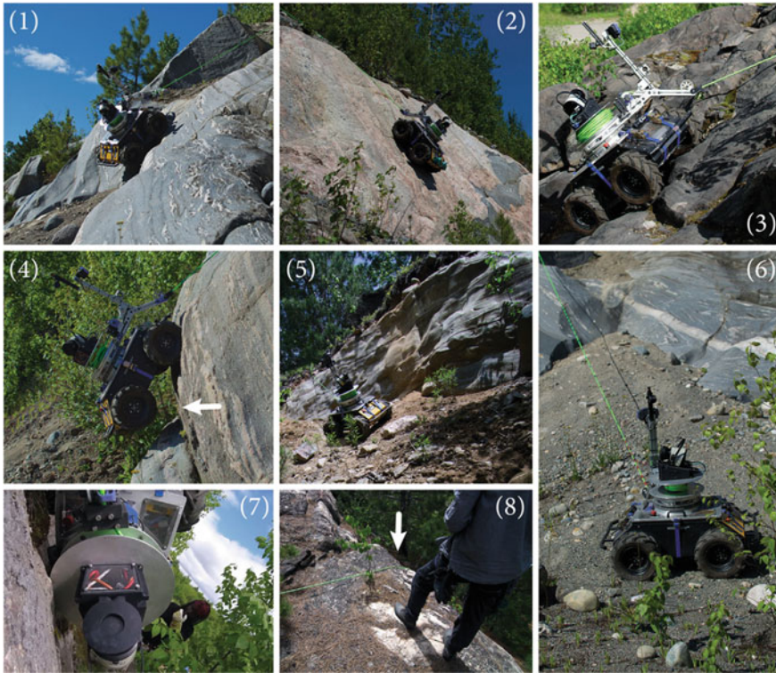
Fig. 14 Platform Evaluation : TReX’s advanced mobility on steep terrain is demonstrated through visual examples during the field deployment. Images 1–3 show TReX successfully navigating steep rock faces. Image 4 shows how the robot’s front tires can lift off the rock due to excessive slope and high tension on the tether. Images 5–6 show the lateral mobility of the robot while under tension. Image 7 shows TReX just after tipping over, which was caused by platform instability when navigating tangent to an angled surface. Image 8 illustrates a common limitation of using a tether; when the taut tether contacts rock, abrasion or severe bending can result in damage
