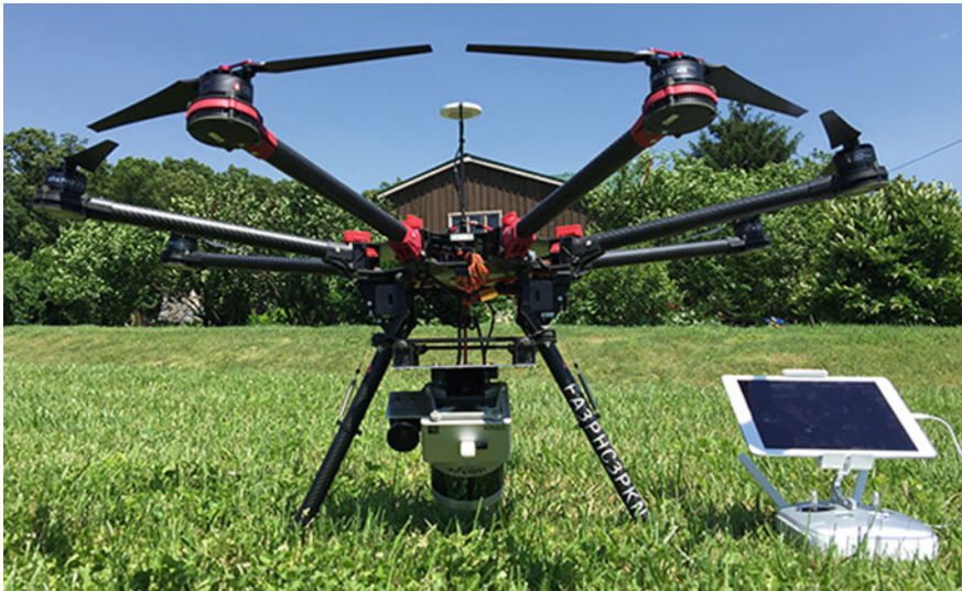
Fig. 9 DJI S1000 aircraft with sensor pack. The aircraft is built with a GPS receiver (on top of the aircraft). GPS data is not used in mapping or autonomous missions as in this paper
