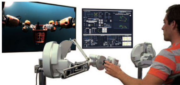
Fig. 2 Pilot Interface. The pilot's interaction with O 2 is established through an immersive interface consisting of bimanual haptic devices, stereoscopic live vision, GUI and a world display giving a global perspective of the scene
