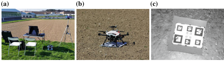
Fig. 2 a Shows our experimental set-up on the field, with the GPS RTK base station visible on the right. b Depicts the AscTec Firefly positioned on the landing platform. c Exemplifies the tag arrangement on the platform as seen by the on-board camera
