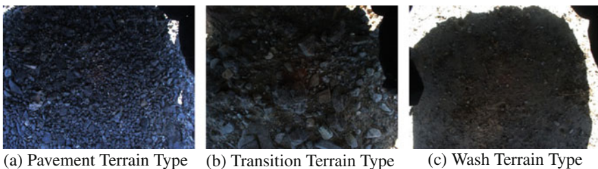
Fig. 4 Different types of terrain in the MVP test area. Pavements were found to be associated with high NSS counts, while washes had low NSS counts. The transition terrain was in between washes and pavements and had moderate NSS counts.
