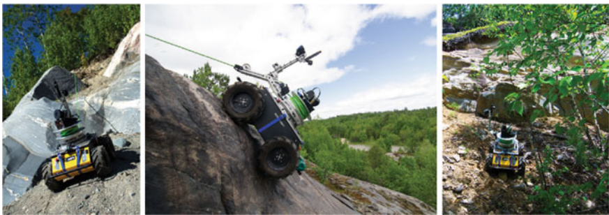
Fig. 1 TReX Field Deployment : Our tethered mobile robot navigates extremely steep terrain in order to generate a 3D map of a spanning rock outcrop that is partially occluded by vegetation. The experiment, which was conducted over several days in an open-pit mine in Northern Ontario, Canada, involved just over 1 km of driving on extremely steep terrain. TReX is anchored at the top of the cliff and manually piloted. The attached electromechanical tether (bright green) provides support, off-board power, and wired communications between the robot and base station
