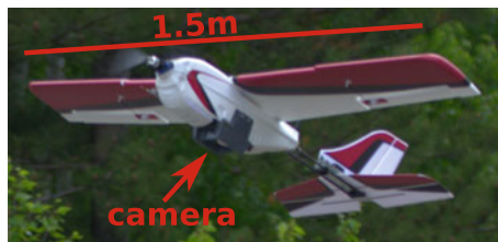
Fig. 1 The PrecisionHawk Lancaster fixed-wing UAV used in experiments, seen here during take-off. Note the payload bay in the centre of the fuselage housing the downward-looking camera used for experiments. (Image: François Pomerleau)
