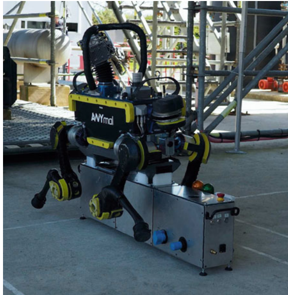
Fig. 7 ANYmal in seated configuration on the docking station at the ARGOS challenge
