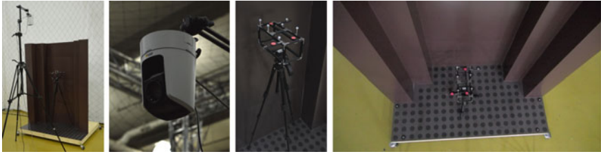
Fig. 6 Subscale mockup system: (far left) experimental setup shown with the subscale mockup of a reactor pressure vessel; (middle left) external camera; (middle right) subscale mockup of the inspection robot; (far right) image of the subscale system from the external camera. Note the complete lack of visual texture on the structure
