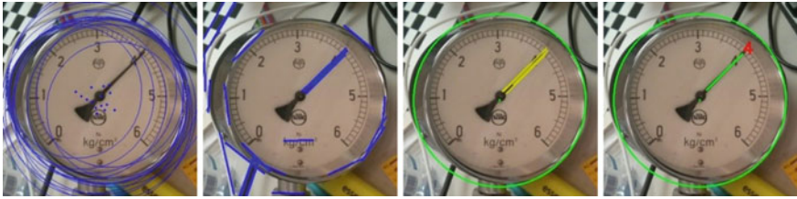
Fig. 11 Pressure gauge reading process (from left to right): (1) multiple circle detections, (2) line segment extractions, (3) resulting mean circle with estimated manometer center (green point) and filtered lines (yellow), (4) mean pointer line (green) and resulting read value in red
