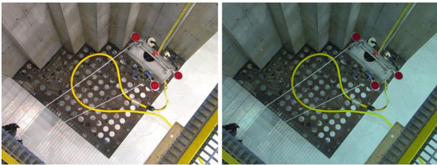
Fig. 8 External camera images from platform testing: (left) clean and (right) degraded with artificial environmental image effects (speckling and color attenuation)
