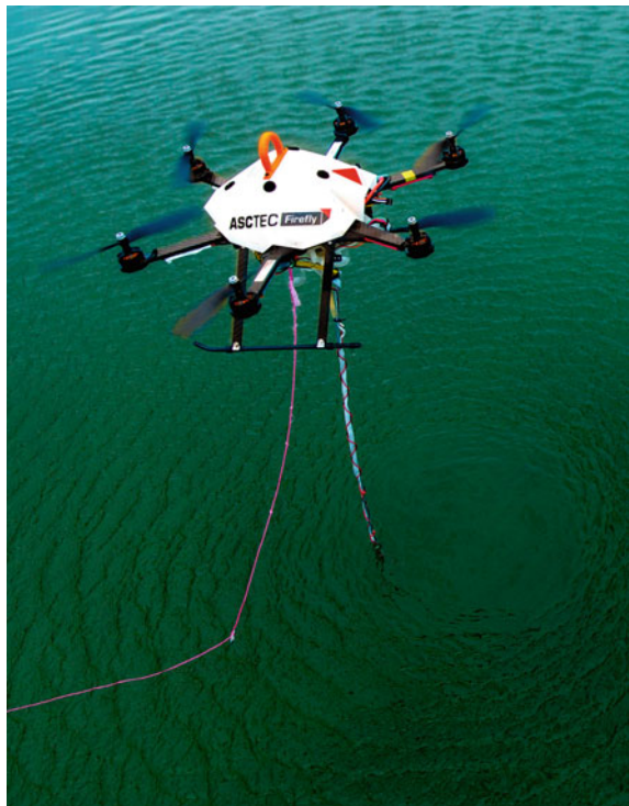
Fig. 1 UAV-system with a passive cable and sensors for measuring water properties at precise depths
