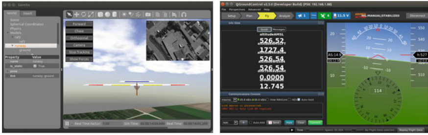
(a) Fixed-wing UAV and synthetic image. (b) Output of QGroundControl in HIL mode.
