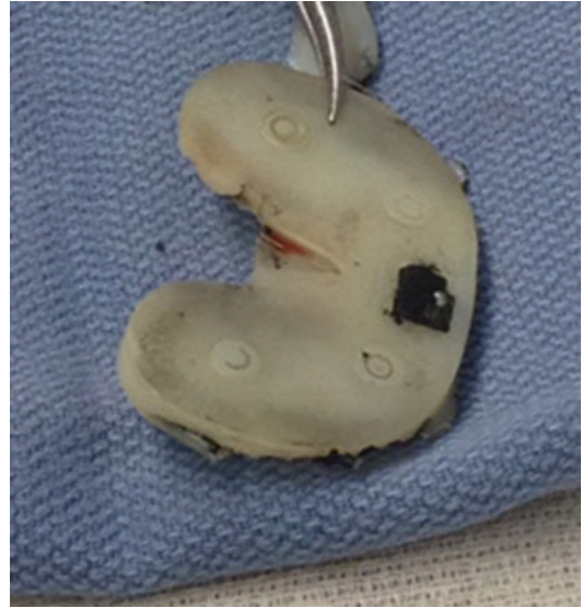
Fig. 25.3. Thinning of the polyethylene insert is seen with backside wear at the posterior locking mechanism
