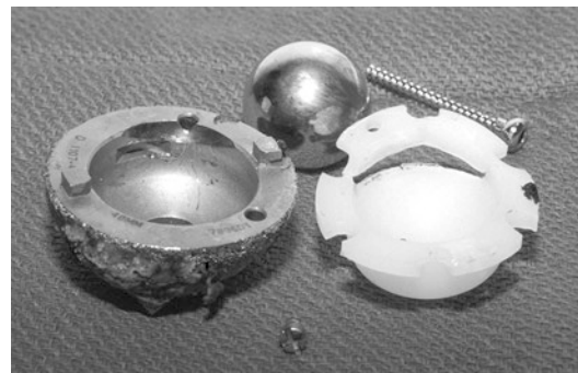
Fig. 2.11 A 1-year conventional UHMWPE, primary acetabular liner demonstrating crack initiation and propagation. Failure initiated at a sharp edge of a locking point (from Tradonsky S, Postak PD, Froimson AI, et al. A comparison of disassociation strength of modular acetabular components. Clin Orthop Relat Res. 1993;296:154–160, with permission)
