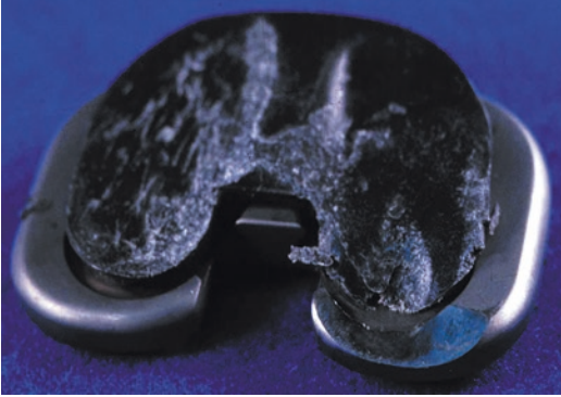
Fig. 2.1 A 5-year retrieval of a failed poly-II tibial insert demonstrating a high component wear rate with infiltration of carbon fibers and polyethylene debris into surrounding tissue
